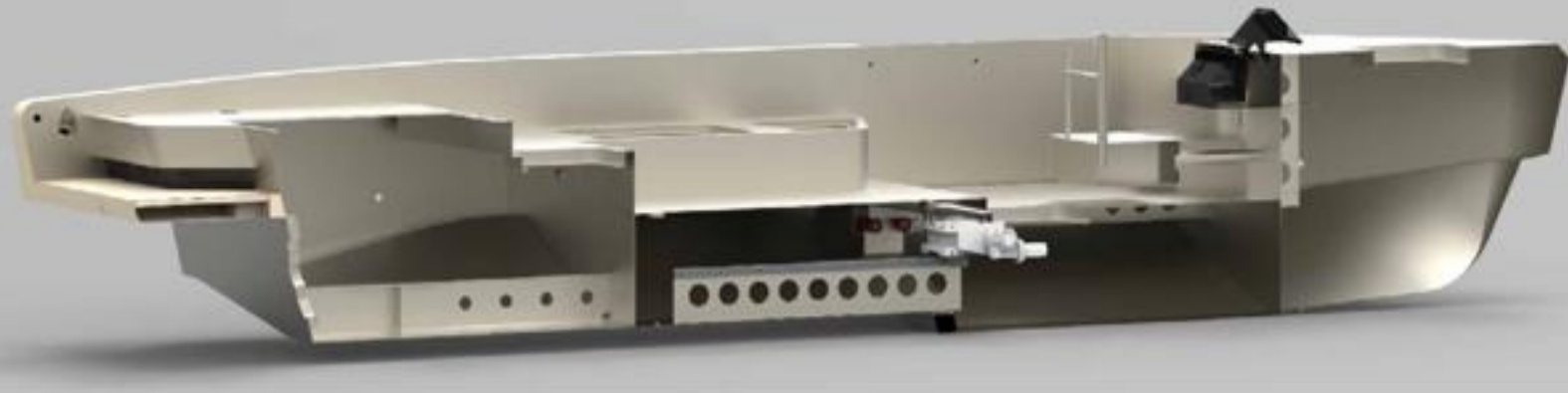
Fig. 2: Perspective view in longitudinal section with the telescopic rack mechanism that makes it possible to lengthen or shorten the boat (Bresciani and PGYD Archive)
